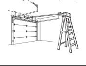
**4.2** Fully open the door and place a 2x4 (laid flat) under the rail. For one-piece doors without tracks, lay the 2x4 on it's side.
